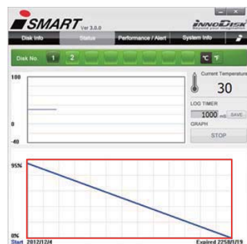
The Life span graph helps user understand the expiry date of Innodisk own's products
